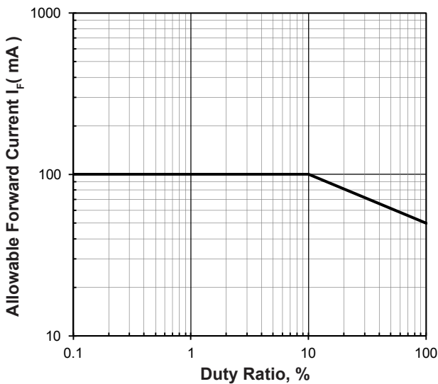
Allowable Forward Current Vs Duty Ratio
